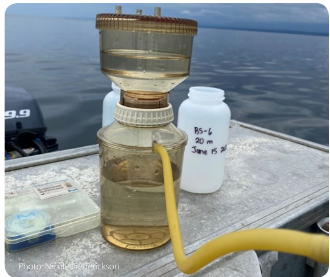
Water samples collected from small vessels are filtered on board using a filter holder and vacuum pump.
